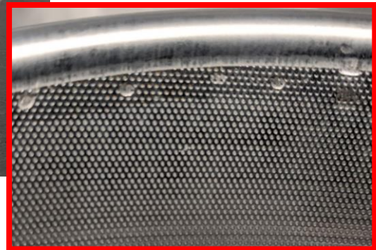
Enlarged view of SB960 hole pattern.
